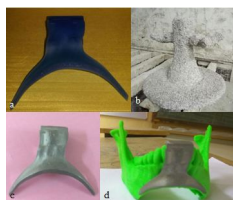
Figure 7: (a) SLA pattern; (b) ceramic mold; (c) SS316 surgical template; (d) metal template and FDM mandible.
